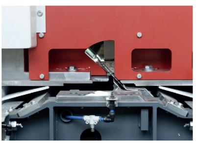
Thanks to the massive steel construction of the machine table, it is possible to use smaller saw blade diameters.
